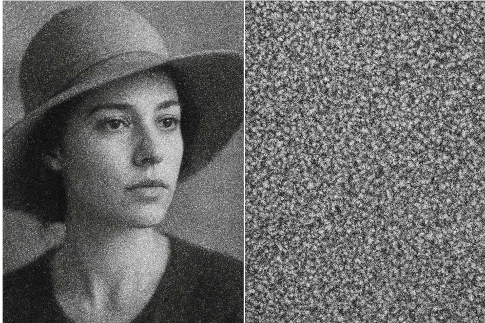
Comparison of enlargements in analog photography. Left: portrait obtained on film with visible grain. Right: enlarged detail of the photosensitive emulsion, revealing the structure of silver-halide crystals responsible for image formation.
